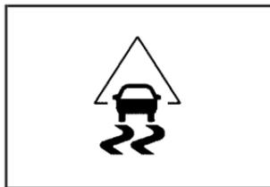
If the vehicle has StabiliTrak<sup>®</sup> this warning light should come on briefly when the ignition is in ON/RUN.
