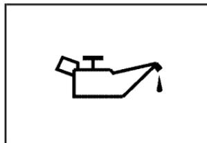
This light will come on briefly as a check to be sure it works, when the ignition is in ON/RUN. If it does not, have your vehicle serviced.
